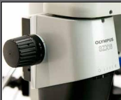
The parfocality of the LCF3 minimizes the need for constant refocusing by the examiner while changing magnification settings. All visual magnifications are clearly marked on the zoom knobs, eliminating the need for use of multipliers to determine the total viewed magnification. A N.I.S.T. traceable Certificate of Magnification Matching is provided with every system at the time of installation.
